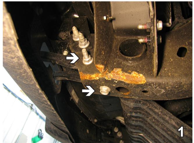
1. Using the 18MM socket, go up in behind to remove the bottom two metric bolts from the tow hook. Do this to both sides of the vehicle. Pull the tow hook forward and set aside. **The tow hooks will not be reinstalled.**
